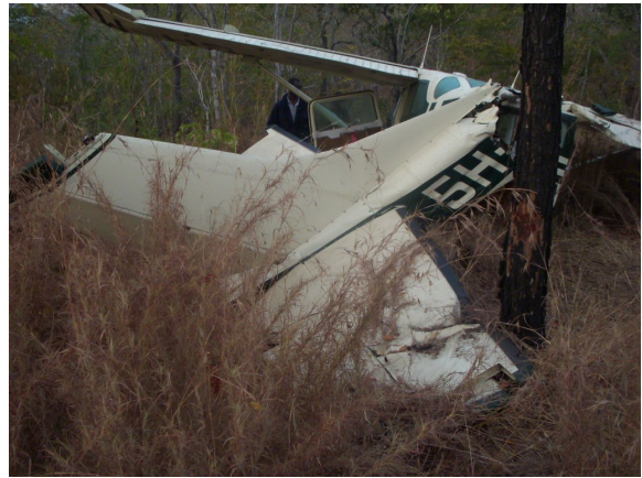
Tail section – note damage to horizontal stabilizer
